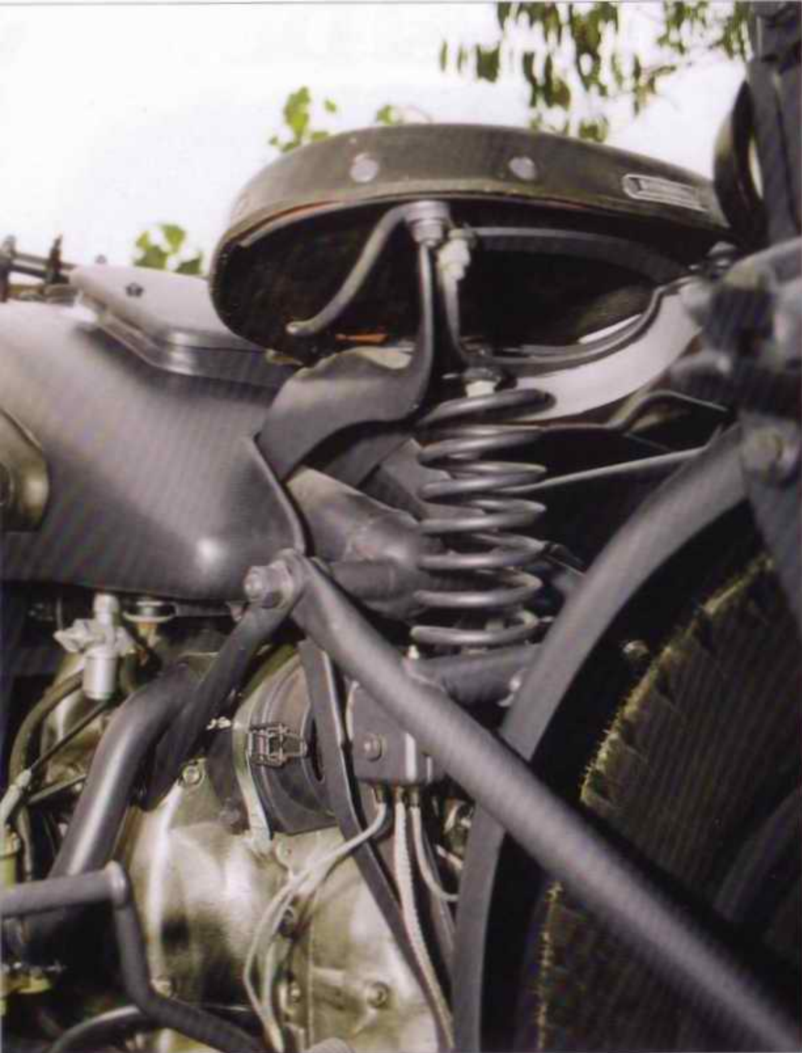
Details and overall view of drivers seat, its fixing with the frame, one oversized spring. On opposite page different type of drivers seat on later model of R 75.
