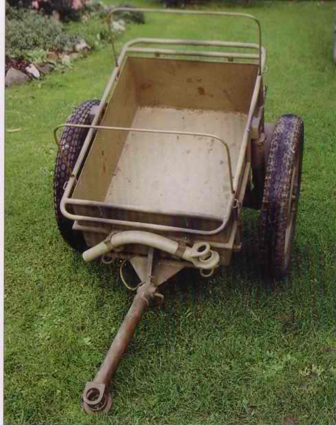
Various manufacturers produced the infantry trailers. They differed mainly in size, frame type and use of wheels - either full metal or with holes. This particular trailer is equipped with construction for canvas. For illustration two trailers are attached to the BMW R 75.
