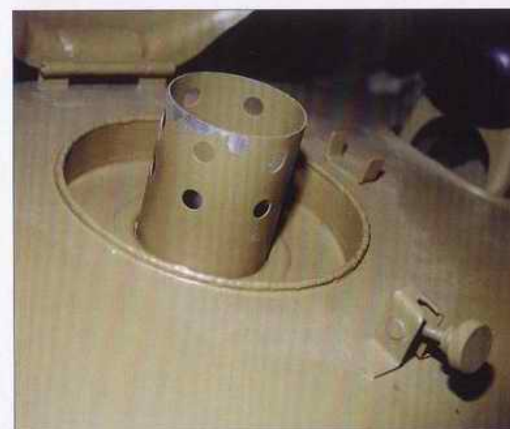
Above closed air filter cover from the front, below folded. On the right - details of intake pipe after filter was taken out. Opening in pipe fit the openings in the center pipe of the filter (below right).
