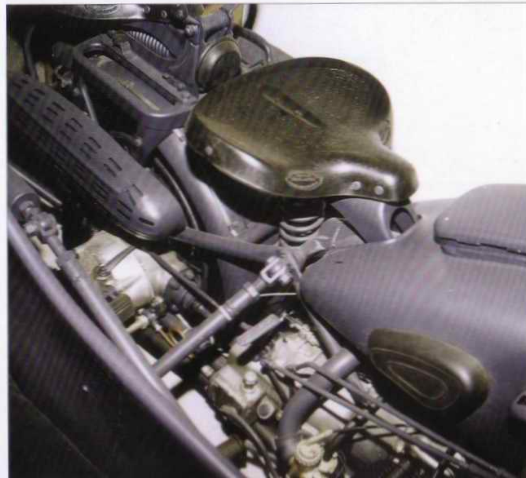
Details and overall view of drivers seat, its fixing with the frame, one oversized spring. On opposite page different type of drivers seat on later model of R 75.
