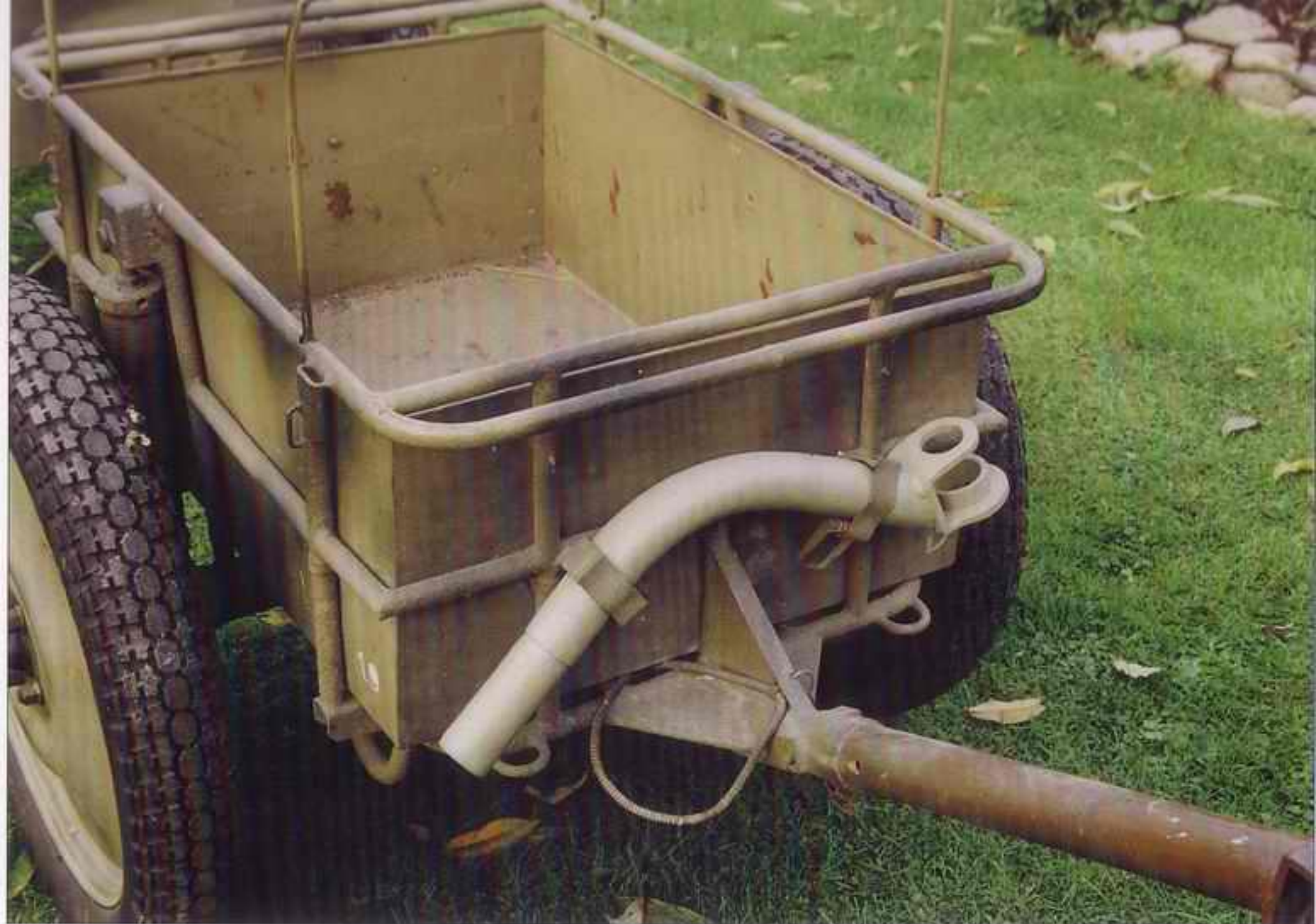
Various manufacturers produced the infantry trailers. They differed mainly in size, frame type and use of wheels - either full metal or with holes. This particular trailer is equipped with construction for canvas. For illustration two trailers are attached to the BMW R 75.
