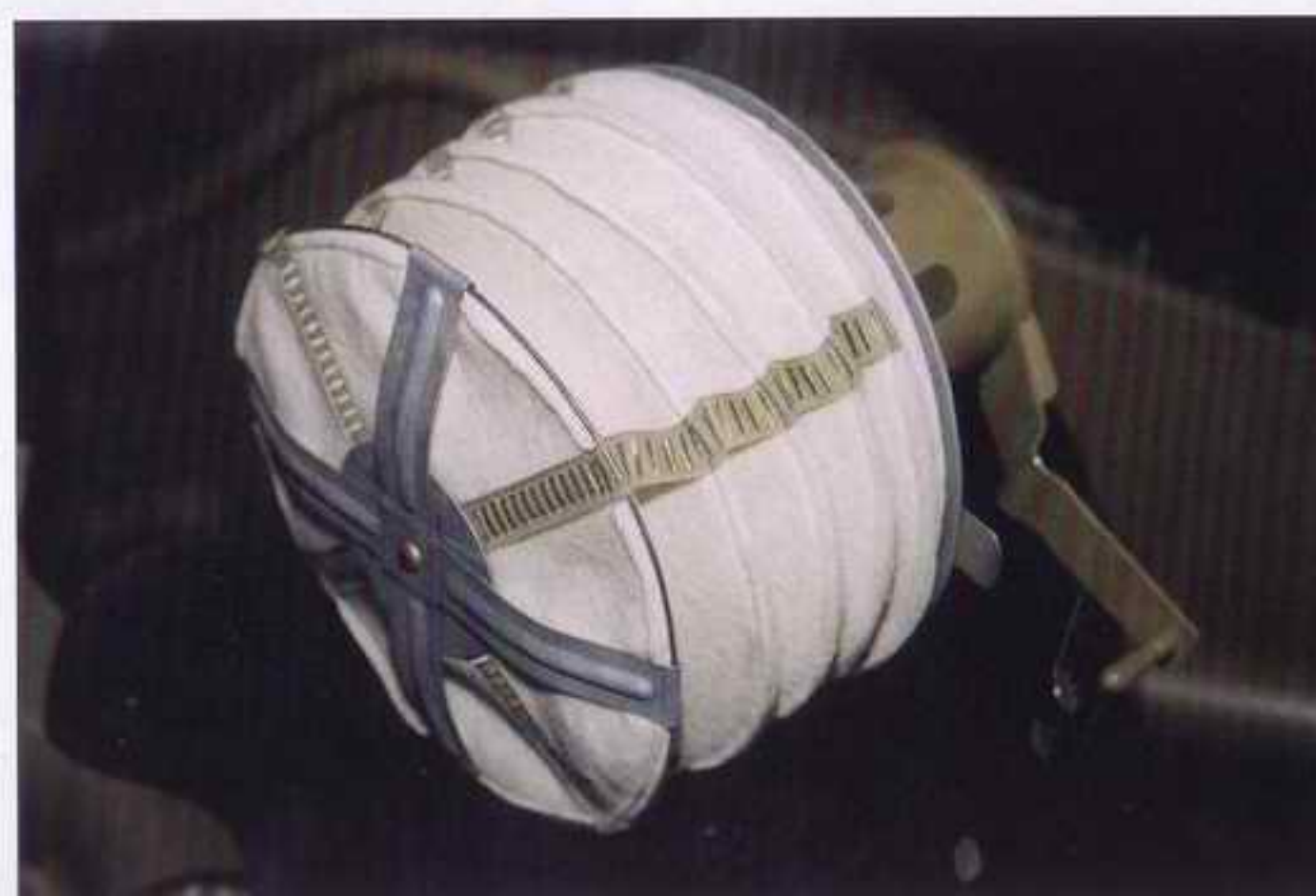
Above closed air filter cover from the front, below folded. On the right - details of intake pipe after filter was taken out. Opening in pipe fit the openings in the center pipe of the filter (below right).
