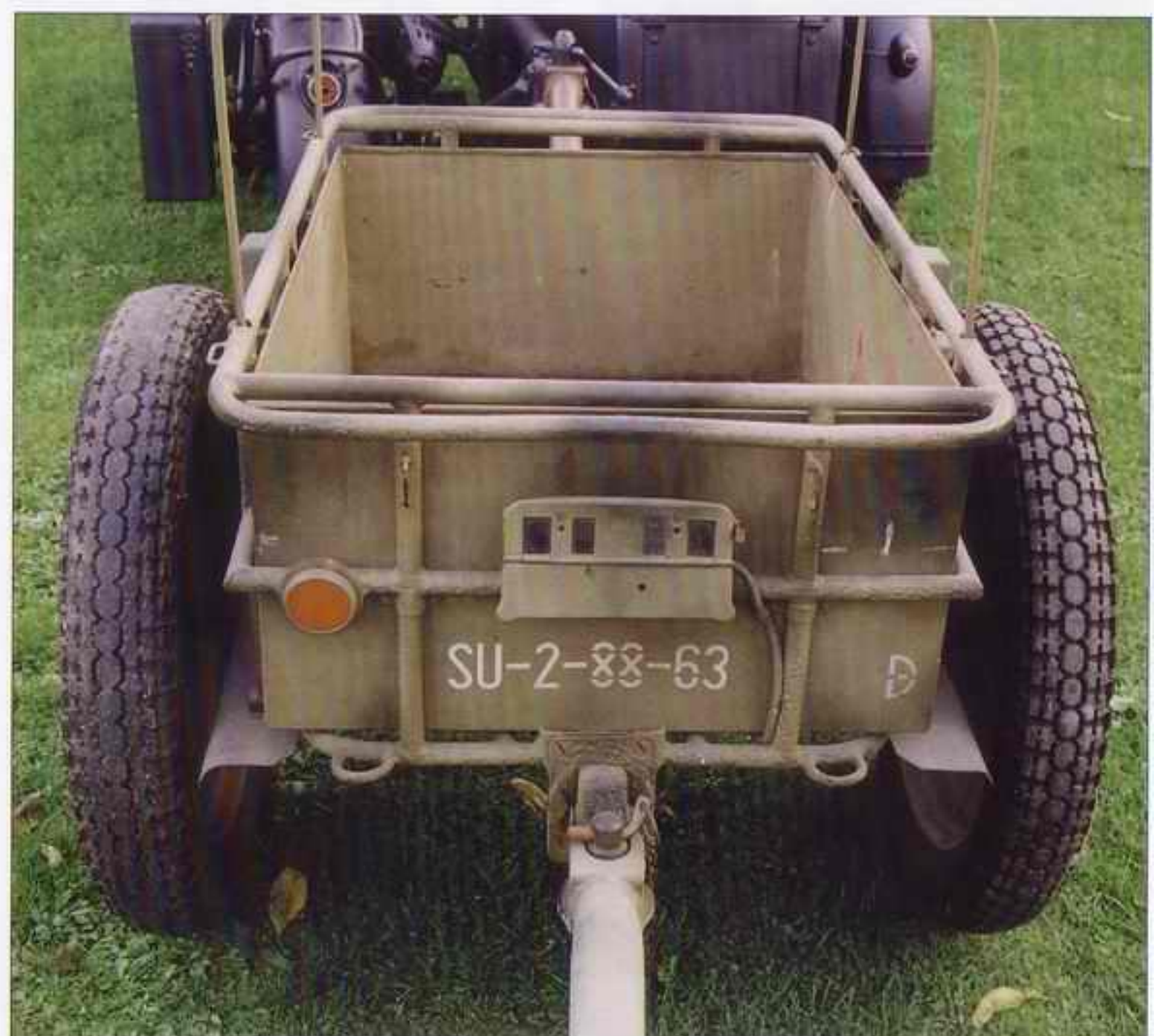
Various manufacturers produced the infantry trailers. They differed mainly in size, frame type and use of wheels - either full metal or with holes. This particular trailer is equipped with construction for canvas. For illustration two trailers are attached to the BMW R 75.
