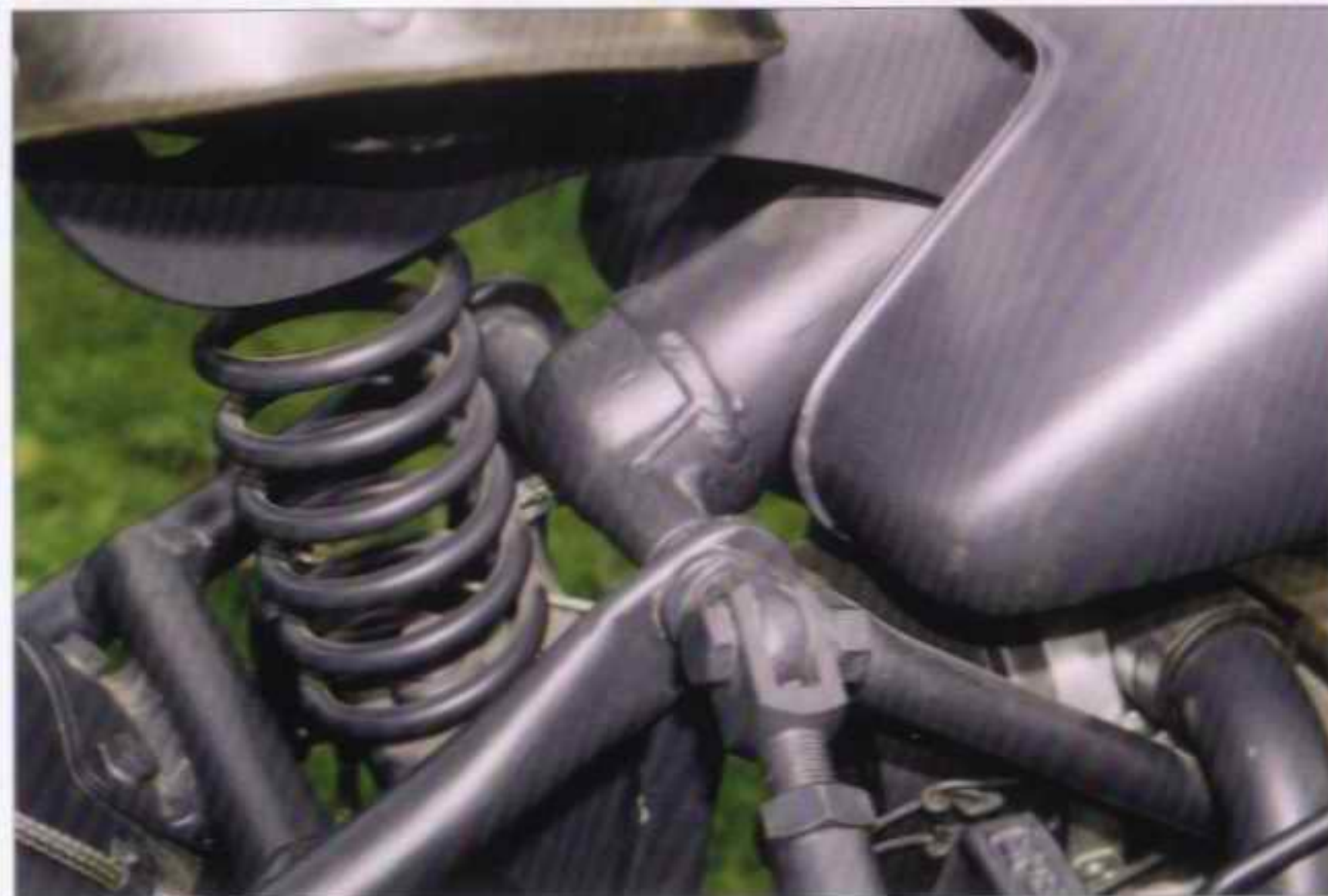
Details and overall view of drivers seat, its fixing with the frame, one oversized spring. On opposite page different type of drivers seat on later model of R 75.
