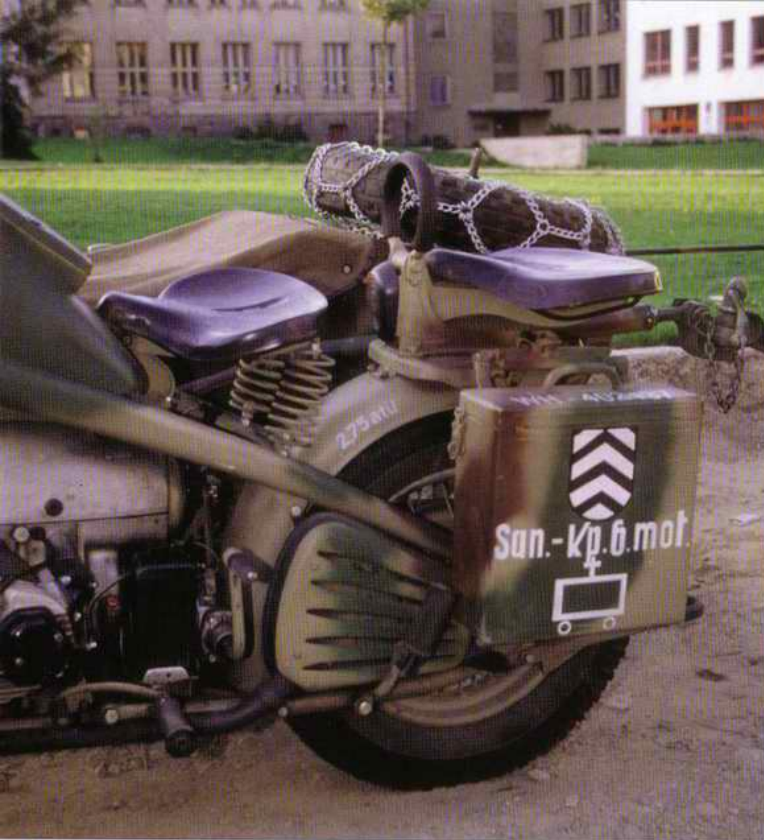
Swinging co-driver's seat was equipped with two upright springs. Co-drivers seat was fixed via two holders and vertical spring - photo below left.
