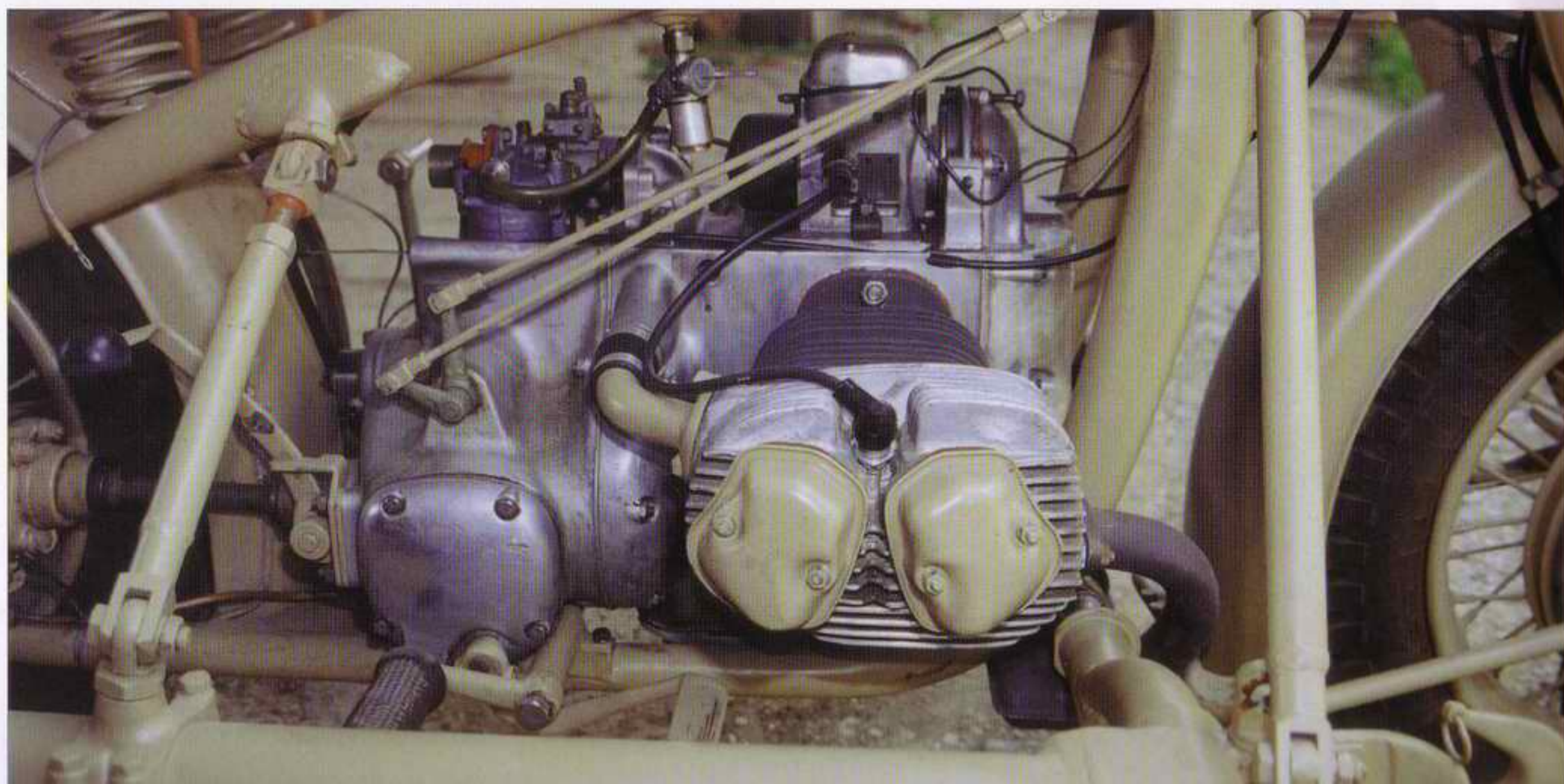
Right side engine view - cylinder equipped with simplified metal covers of valve mechanism from later production models. Engine has the cover off. Extreme left before fender there is a handle for differential locking. In front of handle - brake fluid container with filling cup. In front of foot rest - foot brake handle.
