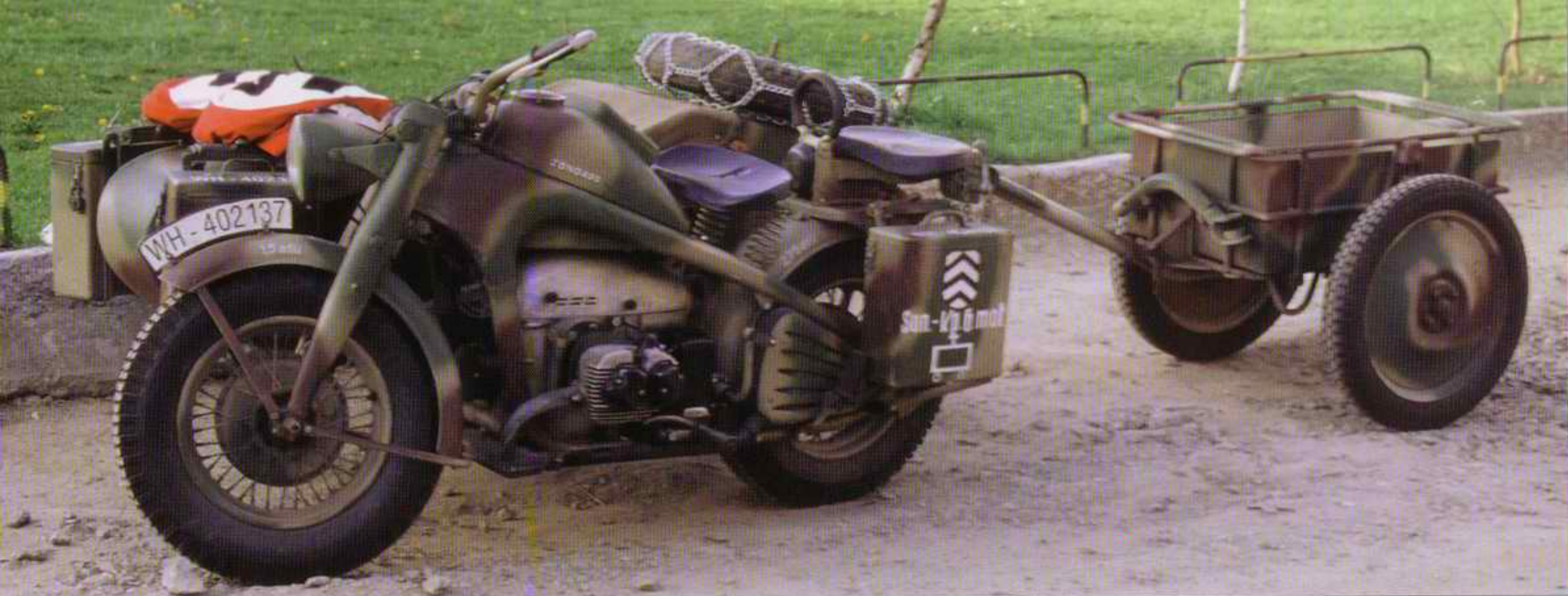
Some motorcycles were equipped with towing device used for towing a Trailer. Frame of the sidecar BW 43 on opposite side shows BMW R 75 type.
