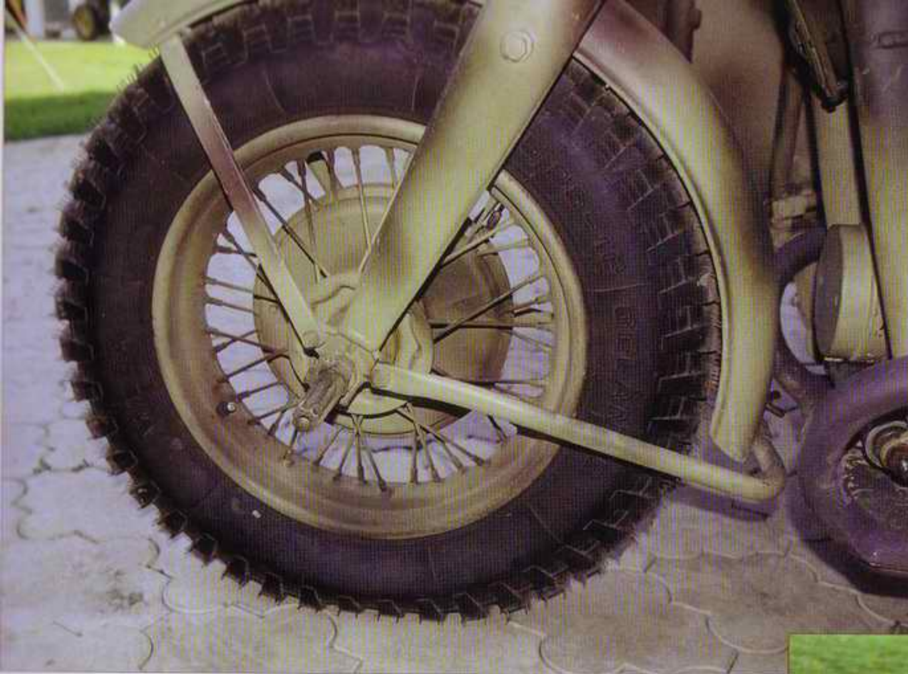
3,00D X 16 front wheel with 4,5 x 16 tyre. The wheel has mechanical drum brakes. 1.5 Atu inscription indicating tyre pressure prescribed.
