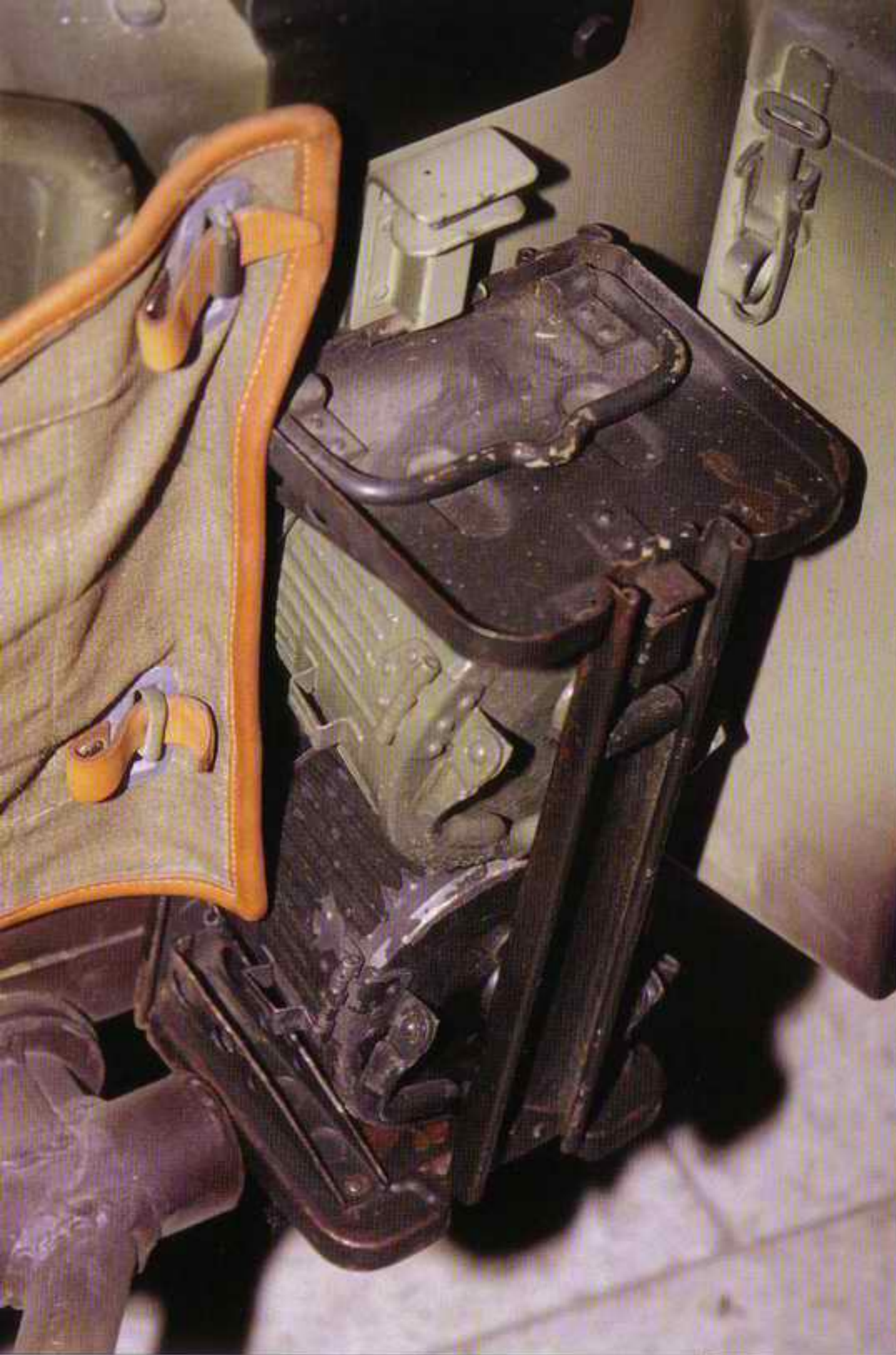
The most famous manufacturer of sidecars was Steib company. All motorcycles were equipped with three map bags on sides of a sidecar. Third was located on left side of a motorcycle behind second seat. First series used leather bags, later metal bags were used.
