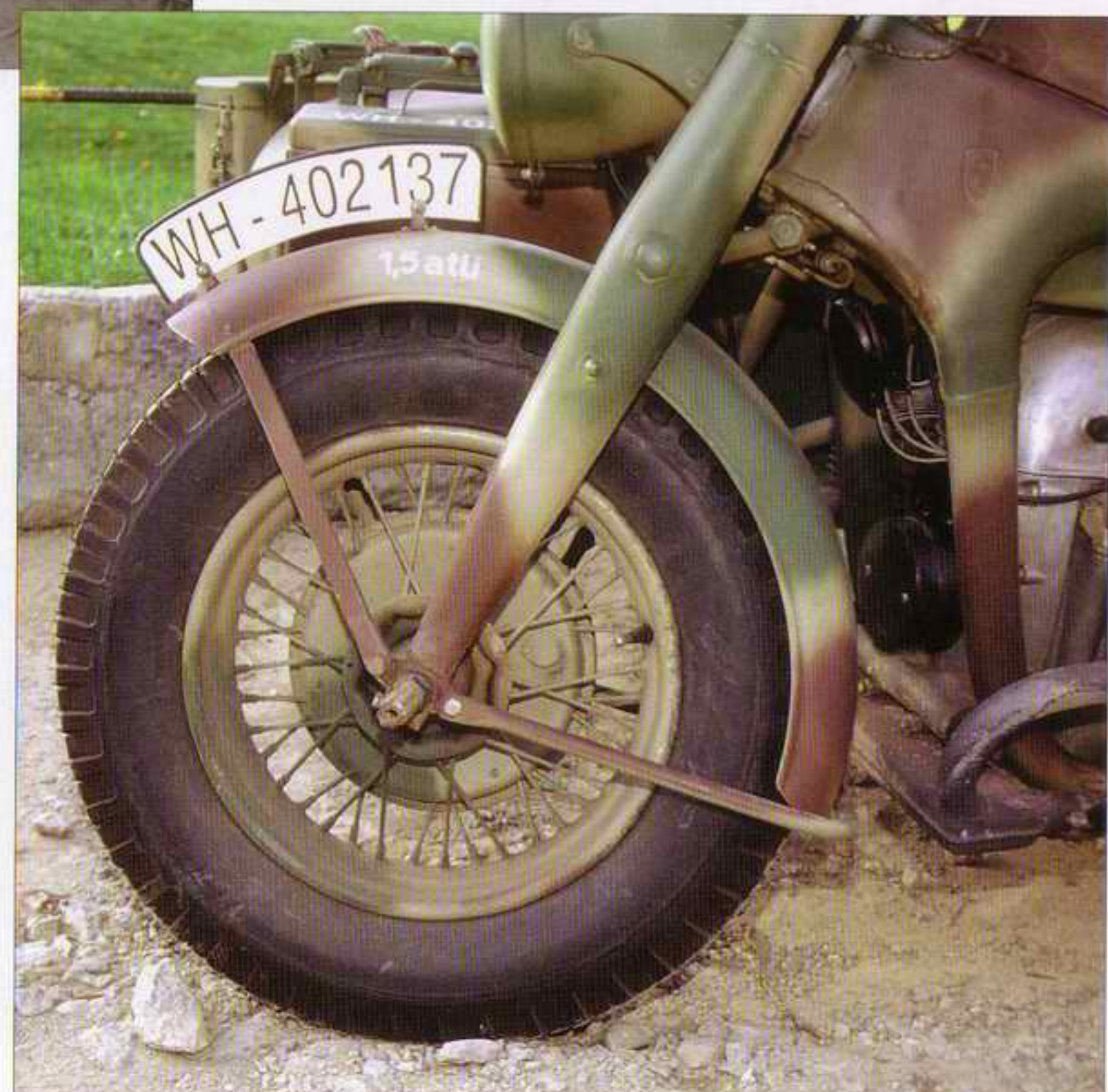
3,00D X 16 front wheel with 4,5 x 16 tyre. The wheel has mechanical drum brakes. 1.5 Atu inscription indicating tyre pressure prescribed.
