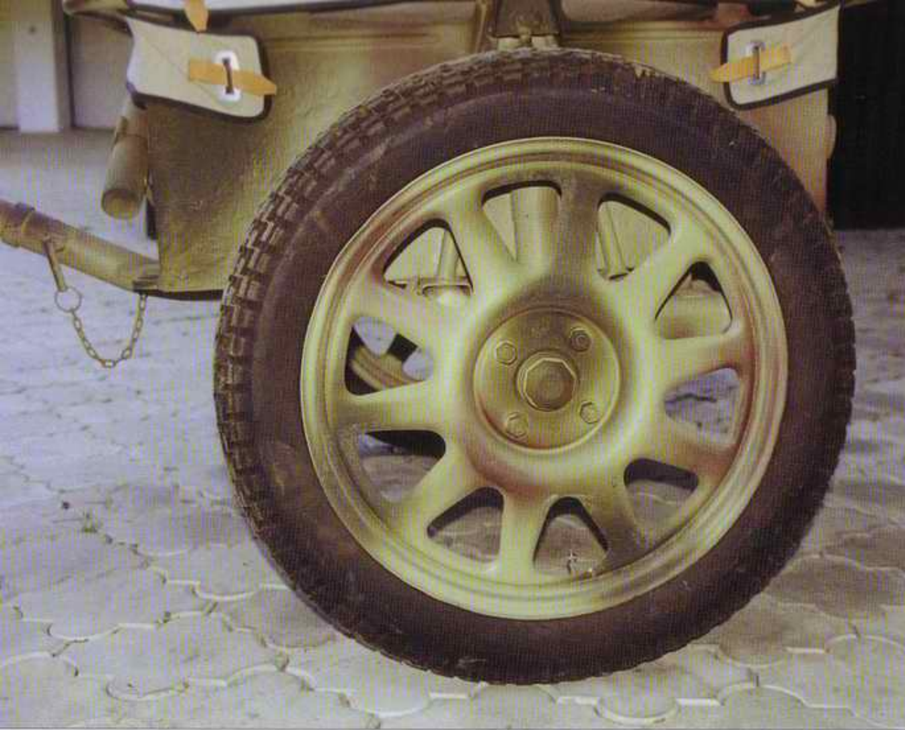
Various manufacturers used different running wheels either with holes or full pressed metal. Trailers were canvas covered.
