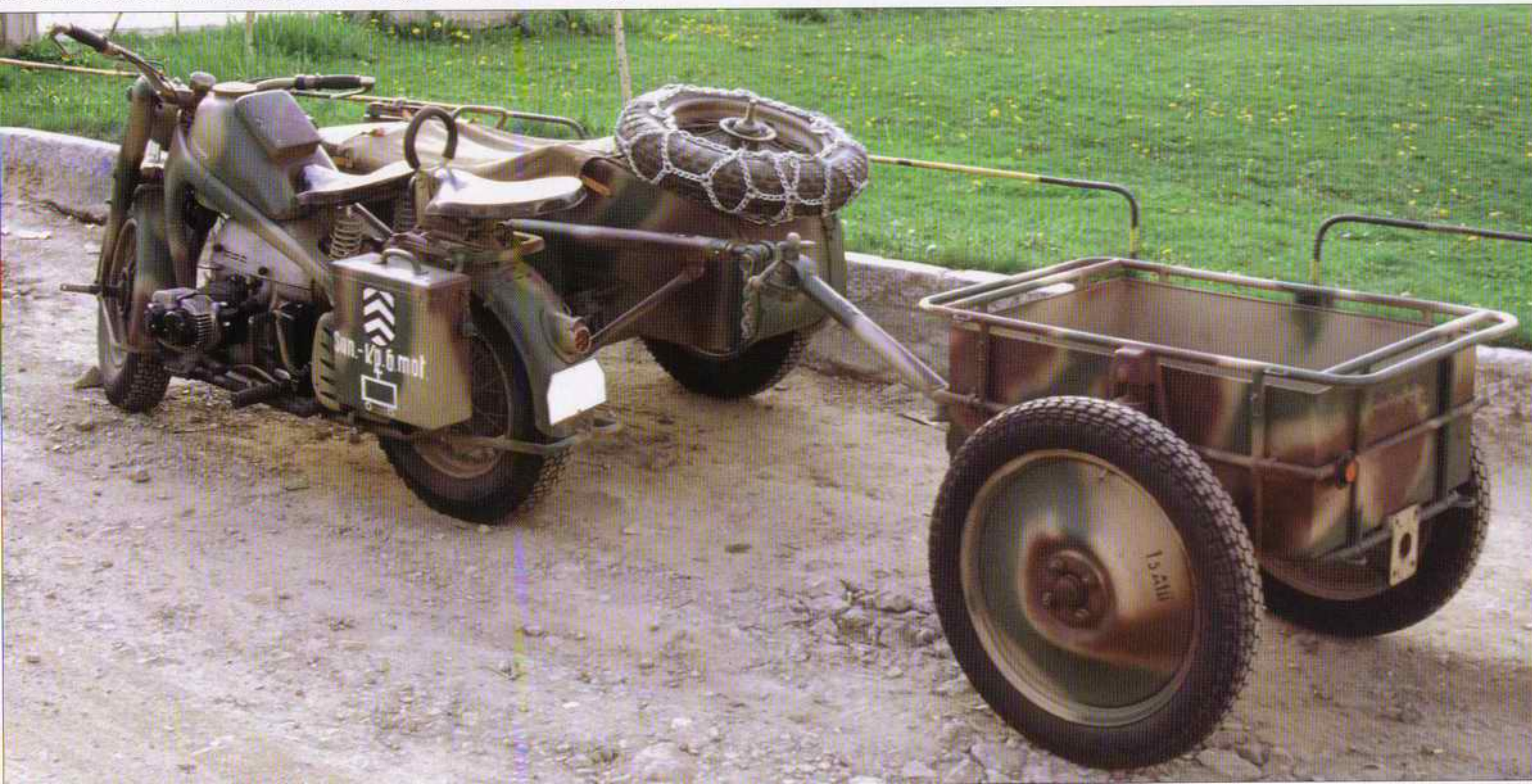
Some motorcycles were equipped with towing device used for towing a Trailer. Frame of the sidecar BW 43 on opposite side shows BMW R 75 type.
