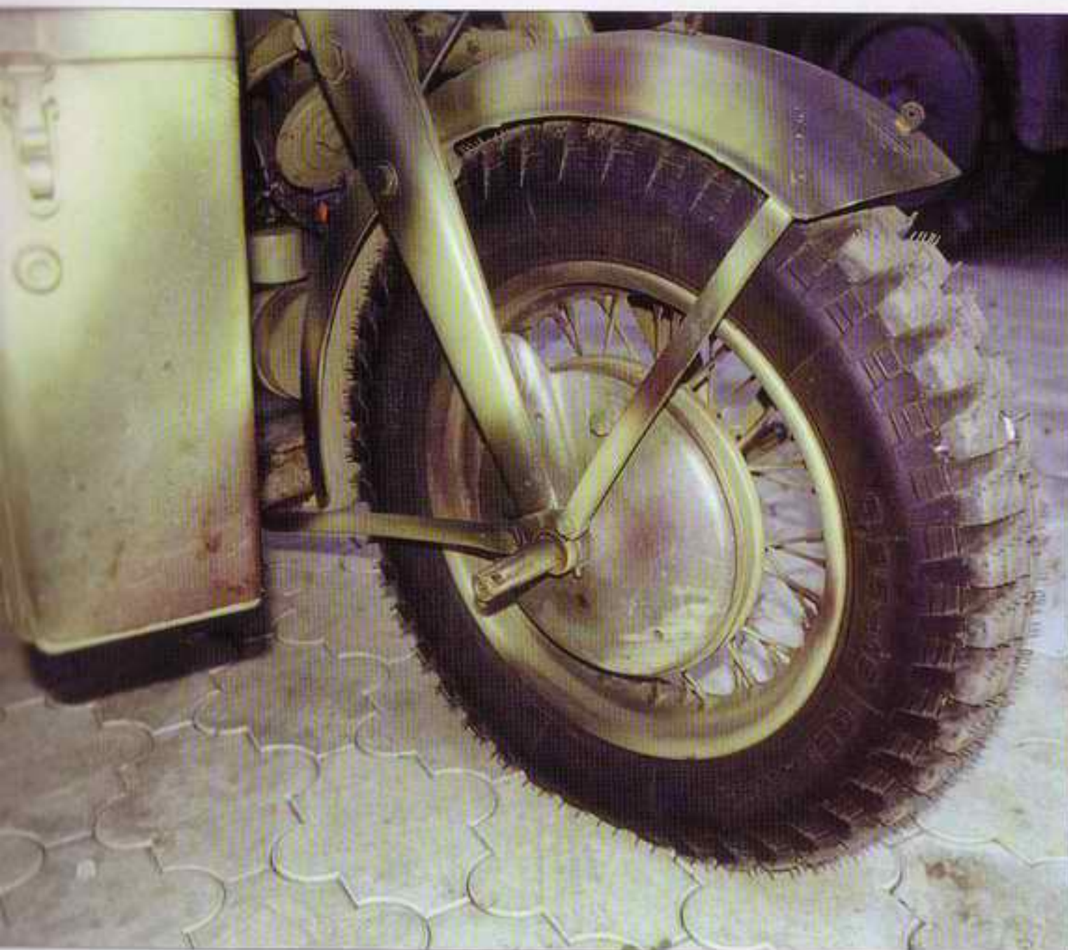
3,00D X 16 front wheel with 4,5 x 16 tyre. The wheel has mechanical drum brakes. 1.5 Atu inscription indicating tyre pressure prescribed.
